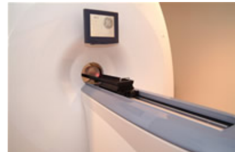
GE Locus Ultra microCT scanner suitable for dynamic preclinical CT imaging with 150 um resolution
