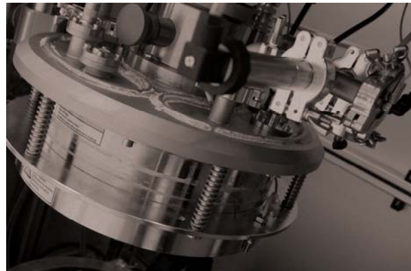
A close-up view of the embossing chamber showing the pressure/heating plate combination, capable of temperatures up to 220°C and forces up to 200kN.
